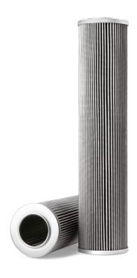
End 2 OD 96.27 mm **Largest OD** 96.27 mm 427.74 mm Length 55.37 mm End 1 ID TWA MICRON @ BETA=2 3 micron TWA MICRON @ BETA=20 7.5 micron TWA MICRON @ BETA=200 12 micron TWA MICRON @ BETA=75 9.5 micron
