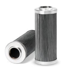
Length 172.97 mm End 1 ID 34.04 mm Largest OD 69.60 mm End 2 OD 69.60 mm TWA MICRON @ BETA=2 3 micron TWA MICRON @ BETA=20 7.5 micron TWA MICRON @ BETA=200 12 micron TWA MICRON @ BETA=75 9.5 micron
