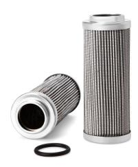
End 2 OD 44.45 mm Largest OD 45.21 mm 113.54 mm Length End 2 ID 24.89 mm TWA MICRON @ BETA=2 3 micron TWA MICRON @ BETA=20 7.5 micron TWA MICRON @ BETA=200 12 micron TWA MICRON @ BETA=75 9.5 micron
