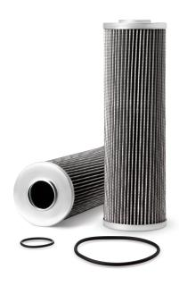
End 1 ID 32.26 mm **Largest OD** 73.66 mm Length 235.97 mm End 2 OD 73.66 mm TWA MICRON @ BETA=2 1 micron TWA MICRON @ BETA=20 3 micron TWA MICRON @ BETA=200 6 micron TWA MICRON @ BETA=75 4.5 micron
