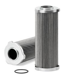
Length 206.50 mm Largest OD 82.55 mm End 1 ID 37.85 mm End 2 OD 81.03 mm TWA MICRON @ BETA=2 1 micron TWA MICRON @ BETA=20 3 micron TWA MICRON @ BETA=200 6 micron TWA MICRON @ BETA=75 4.5 micron
