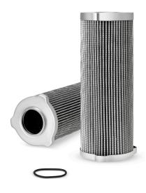
82.55 mm Largest OD End 2 OD 81.03 mm Length 206.50 mm End 1 ID 37.85 mm TWA MICRON @ BETA=2 1 micron TWA MICRON @ BETA=20 3 micron TWA MICRON @ BETA=200 6 micron TWA MICRON @ BETA=75 4.5 micron
