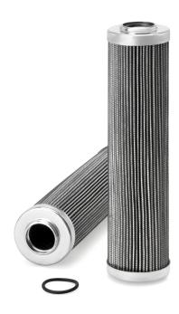
End 2 OD 50.29 mm Length 208.53 mm End 1 ID 23.37 mm Largest OD 50.29 mm TWA MICRON @ BETA=2 1 micron TWA MICRON @ BETA=20 3 micron TWA MICRON @ BETA=200 6 micron TWA MICRON @ BETA=75 4.5 micron
