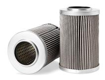
End 2 ID 42.42 mm 116.84 mm Length **Largest OD** 79.25 mm 78.99 mm End 2 OD TWA MICRON @ BETA=2 1 micron TWA MICRON @ BETA=20 3 micron TWA MICRON @ BETA=200 6 micron TWA MICRON @ BETA=75 4.5 micron
