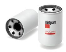
**Largest OD** 93.47 mm **BPV OPENING DP** 0 kPa 1 1/2-16 UN-2B **Thread Size** 147.83 mm Length Seam OD 94.49 mm **Gasket Inside Diameter** 75.44 mm **Gasket OD** 87.63 mm **Standpipe** NO TWA MICRON @ BETA=2 3 micron TWA MICRON @ BETA=20 7.5 micron TWA MICRON @ BETA=200 12 micron TWA MICRON @ BETA=75 9.5 micron
