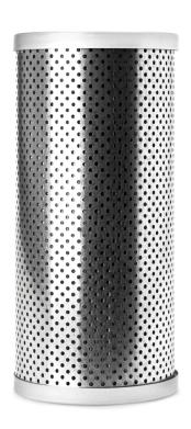
End 2 OD 100.08 mm **BPV OPENING DP** 0 kPa 100.08 mm Largest OD Length 209.80 mm End 2 ID 59.18 mm End 1 ID 59.18 mm TWA MICRON @ BETA=2 4 micron TWA MICRON @ BETA=20 9 micron TWA MICRON @ BETA=75 10 micron
