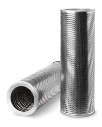
End 1 ID 109.98 mm End 2 ID 109.98 mm Largest OD 150.11 mm Length 453.90 mm End 2 OD 150.11 mm TWA MICRON @ BETA=2 4 micron TWA MICRON @ BETA=20 9 micron TWA MICRON @ BETA=75 12 micron
