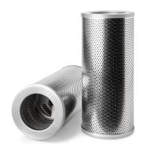
**BPV OPENING DP** 0 kPa End 2 OD 129.54 mm Length 292.10 mm End 2 ID 85.09 mm 129.54 mm Largest OD End 1 ID 85.09 mm TWA MICRON @ BETA=2 4 micron 9 micron TWA MICRON @ BETA=20 TWA MICRON @ BETA=75 10 micron
