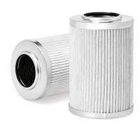
42.42 mm End 2 ID 79.25 mm Largest OD 78.99 mm End 2 OD 0 kPa **BPV OPENING DP** 117.60 mm Length TWA MICRON @ BETA=2 1 micron TWA MICRON @ BETA=20 6 micron TWA MICRON @ BETA=200 14 micron TWA MICRON @ BETA=75 11 micron
