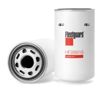
Largest OD 128.00 mm 228.00 mm Length **BPV OPENING DP** Yes **Thread Form** British **Gasket Inside Diameter** 97.00 mm **Gasket OD** 107.00 mm 1000 kPa **Hydrostatic Burst Minimum** Particle Size at Beta 75 75 micron Internal Thread Type
