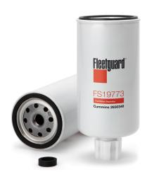
**Thread Size** M16 X 1.5-6H INT 176.28 mm Length 76.45 mm **Largest OD Gasket Inside Diameter** 62.53 mm **Gasket OD** 72.19 mm Seam OD 77.47 mm **Standpipe** NO **EFFICIENCY, TWA BY SAE J 1985** 98.7% **EMULSIFIED WATER SEPARATION** 95% FREE WATER SEPARATION 95% **MICRON RATING BY SAE J 1985** 5 micron
