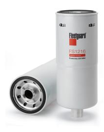
**Thread Size** 1 1/4-12 UNS-2B **Largest OD** 116.10 mm 314.20 mm Length **Gasket Inside Diameter** 96.50 mm Gasket OD 109.70 mm 118.50 mm Seam OD NO **Standpipe** 96% **EFFICIENCY, TWA BY SAE J 1985** 90% **EMULSIFIED WATER SEPARATION** 90% FREE WATER SEPARATION **MICRON RATING BY SAE J 1985** 20 micron
