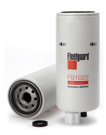
93.83 mm Largest OD 1-14 UNS-2B **Thread Size** 238.30 mm Length StrataPore Media Type **Gasket Inside Diameter** 62.48 mm **Gasket OD** 71.88 mm Seam OD 93.50 mm YES Standpipe 98.7% **EFFICIENCY, TWA BY SAE J 1985 EMULSIFIED WATER SEPARATION** 95% FREE WATER SEPARATION 95% **MICRON RATING BY SAE J 1985** 10 micron
