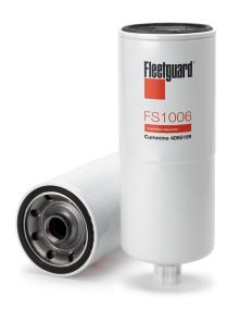
**Thread Size** 1 1/4-12 UNS-2B Length 313.00 mm 116.20 mm **Largest OD Gasket Inside Diameter** 98.20 mm **Gasket OD** 111.40 mm Seam OD 120.29 mm YES Standpipe **EFFICIENCY, TWA BY SAE J 1985** 98.7% **EMULSIFIED WATER SEPARATION** 95 % FREE WATER SEPARATION 95 % **MICRON RATING BY SAE J 1985** 10 micron
