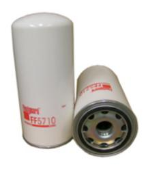
Gasket OD 111.00 mm **Gasket Inside Diameter** 100.00 mm Thread Pitch 1.50 mm **Thread Form** Metric 304.00 mm Length **Thread Diameter** 39.00 mm 140.00 mm Largest OD **Hydrostatic Burst Minimum** 2500 kPa Thread Type Internal **Flow Direction** Outside In **Thread Seal Type** Internal
