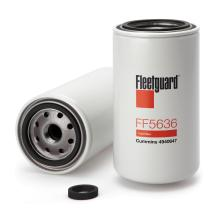
**Gasket Inside Diameter** 62.48 mm **Gasket OD** 71.88 mm Thread Size 7/8-14 UNF-2B Length 175.77 mm 93.47 mm Largest OD Seam OD 93.22 mm NO **Standpipe EFFICIENCY, TWA BY SAE J 1985** 98.7% **MICRON RATING BY SAE J 1985** 5 micron
