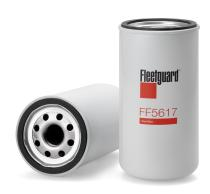
**Gasket Inside Diameter** 62.48 mm 71.88 mm **Gasket OD** 76.45 mm **Largest OD** Length 150.11 mm 7/8-14 UNF-2B **Thread Size** Seam OD 77.83 mm Standpipe NO **EFFICIENCY, TWA BY SAE J 1985** 98.7% **MICRON RATING BY SAE J 1985** 10 micron
