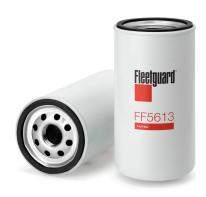
**Gasket OD** 71.88 mm Gasket Inside Diameter 62.48 mm **Largest OD** 76.45 mm **Thread Size** 7/8-14 UNF-2B 150.11 mm Length Seam OD 77.83 mm NO **Standpipe EFFICIENCY, TWA BY SAE J 1985** 98.7% **MICRON RATING BY SAE J 1985** 5 micron
