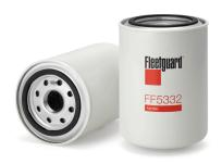
**Gasket OD** 71.88 mm **Gasket Inside Diameter** 62.48 mm Length 137.41 mm 1-14 UNS-2B **Thread Size** Largest OD 93.22 mm 93.98 mm Seam OD **Standpipe** NO **MICRON RATING BY SAE J 1858** 20 micron 99% **EFFICIENCY, TWA BY SAE J 1858**
