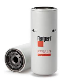
**Gasket OD** 71.88 mm **Gasket Inside Diameter** 62.48 mm 240.54 mm Length **Largest OD** 93.47 mm 1-14 UNS-2B **Thread Size** Seam OD 93.22 mm NO **Standpipe** 98.7% **EFFICIENCY, TWA BY SAE J 1985 MICRON RATING BY SAE J 1985** 5 micron
