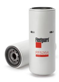
**Gasket Inside Diameter** 62.48 mm **Gasket OD** 71.88 mm 93.47 mm Largest OD Thread Size 1-14 UNS-2B Length 240.54 mm Seam OD 93.22 mm **Standpipe** NO **EFFICIENCY, TWA BY SAE J 1985** 99% **MICRON RATING BY SAE J 1985** 20 micron
