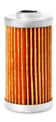
Largest OD35.00 mmLength69.50 mmLargest End ID12.50 mmGasket Inside Diameter11.20 mmFlow DirectionOutside In
