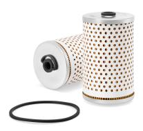
Length145.00 mmLargest OD83.50 mmLargest End ID13.60 mmGasket Inside Diameter13.60 mmFlow DirectionOutside In
