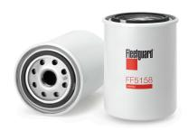
Gasket Inside Diameter 57.40 mm Gasket OD 64.01 mm **Thread Size** 3/4-16 UNF-2B Length 114.05 mm **Largest OD** 80.52 mm 84.33 mm Seam OD NO **Standpipe EFFICIENCY, TWA BY SAE J 1858** 68% **MICRON RATING BY SAE J 1858** 10 micron
