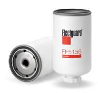
**Gasket Inside Diameter** 62.00 mm **Gasket OD** 70.00 mm Thread Form Metric **Largest OD** 77.00 mm Length 156.00 mm **Thread Diameter** 16.00 mm **Thread Pitch** 1.50 mm **Hydrostatic Burst Minimum** 1500 kPa **Thread Class** 6H **Thread Type** Internal Thread Seal Type Internal
