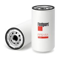
79.25 mm **Gasket Inside Diameter Gasket OD** 88.65 mm 1-14 UNS-2B **Thread Size** Length 175.51 mm 93.22 mm Largest OD Seam OD 93.62 mm NO Standpipe **EFFICIENCY, TWA BY SAE J 1985** 97% **MICRON RATING BY SAE J 1985** 8 micron
