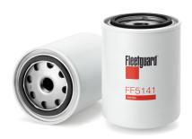
**Gasket OD** 72.14 mm 62.74 mm **Gasket Inside Diameter** Largest OD 93.47 mm 3/4-16 UNF-2B **Thread Size** 127.25 mm Length Seam OD 94.49 mm NO **Standpipe EFFICIENCY, TWA BY SAE J 1858** 96% **MICRON RATING BY SAE J 1858** 20 micron
