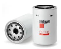
**Gasket Inside Diameter** 62.48 mm **Gasket OD** 71.88 mm **Largest OD** 93.22 mm 1-14 UNS-2B **Thread Size** Length 146.56 mm 93.73 mm Seam OD NO **Standpipe EFFICIENCY, TWA BY SAE J 1858** 50% **MICRON RATING BY SAE J 1858** 20 micron
