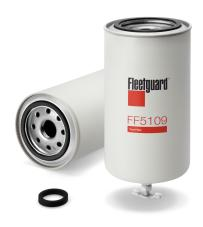
71.88 mm **Gasket OD** 62.48 mm **Gasket Inside Diameter** Largest OD 93.22 mm 196.85 mm Length **Thread Size** 15/16-16 UN-2B Seam OD 93.78 mm NO Standpipe **EFFICIENCY, TWA BY SAE J 1858** 97% **MICRON RATING BY SAE J 1858** 20 micron
