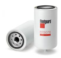
**Gasket Inside Diameter** 62.48 mm **Gasket OD** 71.88 mm **Thread Size** 1-14 UNS-2B 193.04 mm Length Largest OD 93.47 mm Seam OD 94.49 mm NO **Standpipe EFFICIENCY, TWA BY SAE J 1858** 95% **MICRON RATING BY SAE J 1858** 20 micron
