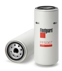
**Gasket OD** 71.88 mm 62.48 mm **Gasket Inside Diameter** 93.73 mm **Largest OD** Length 224.03 mm **Thread Size** 7/8-14 UNF-2B Seam OD 93.22 mm NO **Standpipe EFFICIENCY, TWA BY SAE J 1985** 97% **MICRON RATING BY SAE J 1985** 8 micron
