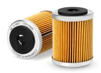
Largest OD51.00 mmLength66.00 mmGasket Inside Diameter13.50 mmGasket OD36.00 mmFlow DirectionOutside In
