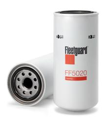
**Gasket OD** 71.98 mm **Gasket Inside Diameter** 62.53 mm 204.72 mm Length **Thread Size** 1-14 UNS-2B 93.47 mm Largest OD Seam OD 94.49 mm **Standpipe** NO **EFFICIENCY, TWA BY SAE J 1858** 99% **MICRON RATING BY SAE J 1858** 20 micron
