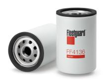
Gasket Inside Diameter62.48 mmGasket OD76.96 mmLength117.60 mmLargest OD76.45 mmThread Size3/4-16 UNF-2B
