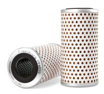
Length5.43 inchLargest End ID1.32 inchLargest OD2.80 inchGasket Inside Diameter1.36 inchGasket OD2.03 inchFlow DirectionOutside In
