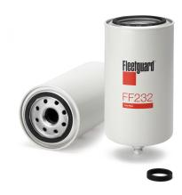
**Gasket Inside Diameter** 62.48 mm 71.88 mm **Gasket OD** Largest OD 93.47 mm **Thread Size** 1-14 UNS-2B 193.04 mm Length Seam OD 94.49 mm NO **Standpipe EFFICIENCY, TWA BY SAE J 1858** 97% **MICRON RATING BY SAE J 1858** 20 micron
