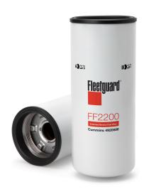
**Gasket Inside Diameter** 78.74 mm 97.00 mm **Gasket OD** 93.98 mm Largest OD **Thread Size** M72 X 2-7H INT 228.19 mm Length Seam OD 95.76 mm NO **Standpipe EFFICIENCY, TWA BY SAE J 1985** 98.7% **MICRON RATING BY SAE J 1985** 15 micron
