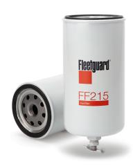
**Thread Size** M16 X 1.5-6H INT Largest OD 76.53 mm Length 171.35 mm **Gasket Inside Diameter** 62.53 mm **Gasket OD** 71.98 mm 77.47 mm Seam OD NO **Standpipe EFFICIENCY, TWA BY SAE J 1858** 97% **MICRON RATING BY SAE J 1858** 20 micron
