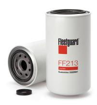
**Gasket Inside Diameter** 62.48 mm **Gasket OD** 71.88 mm 175.51 mm Length **Thread Size** 1-14 UNS-2B 93.22 mm **Largest OD** 95.76 mm Seam OD NO **Standpipe EFFICIENCY, TWA BY SAE J 1858** 96% **MICRON RATING BY SAE J 1858** 20 micron
