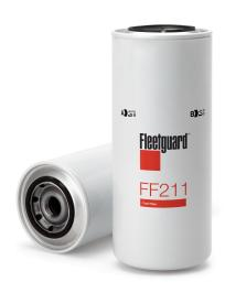
Gasket Inside Diameter 62.59 mm **Gasket OD** 71.63 mm Thread Size 1-14 UNS-2B **Largest OD** 107.67 mm Length 265.05 mm Seam OD 108.20 mm NO Standpipe **EFFICIENCY, TWA BY SAE J 1985** 97%
