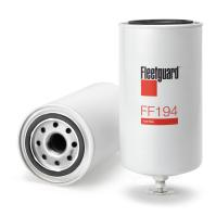
**Gasket OD** 71.37 mm **Gasket Inside Diameter** 62.48 mm **Largest OD** 93.47 mm Length 196.09 mm 1-14 UNS-2B **Thread Size** Seam OD 94.49 mm NO **Standpipe EFFICIENCY, TWA BY SAE J 1858** 97% **MICRON RATING BY SAE J 1858** 20 micron
