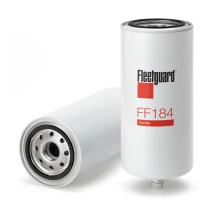
62.48 mm **Gasket Inside Diameter Gasket OD** 71.88 mm **Thread Size** 1-14 UNS-2B Length 223.01 mm 93.22 mm **Largest OD** Seam OD 93.73 mm NO **Standpipe EFFICIENCY, TWA BY SAE J 1858** 85% **MICRON RATING BY SAE J 1858** 20 micron
