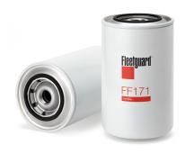
**Gasket Inside Diameter** 62.59 mm 71.63 mm **Gasket OD** 107.67 mm **Largest OD** Length 181.23 mm 7/8-16 UN-2B **Thread Size** Seam OD 108.20 mm NO **Standpipe** 97% **EFFICIENCY, TWA BY SAE J 1858**
