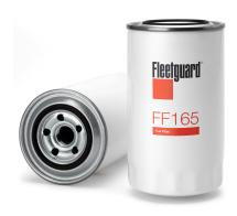
**Gasket OD** 63.00 mm **Gasket Inside Diameter** 55.50 mm Length 162.00 mm 92.50 mm **Largest OD** 20.00 mm **Thread Diameter Thread Form** Metric **Thread Pitch** 1.50 mm **Hydrostatic Burst Minimum** 1500 kPa 6H **Thread Class Thread Type** Internal Flow Direction Outside In Thread Seal Type Internal
