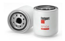
**Gasket Inside Diameter** 62.53 mm Gasket OD 71.98 mm **Thread Size** 1-14 UNS-2B 105.44 mm Length Largest OD 92.96 mm Seam OD 93.98 mm NO **Standpipe EFFICIENCY, TWA BY SAE J 1858** 96% **MICRON RATING BY SAE J 1858** 20 micron
