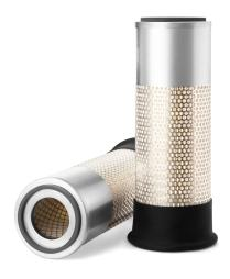
Largest OD Largest ID Flame Resistant Media Flow Direction Type Seal 133.00 mm 68.90 mm No Outside In Axial
